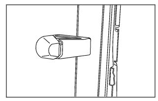
If the vehicle has this feature, squeeze the latch in the center of the window and slide the glass to open it.
